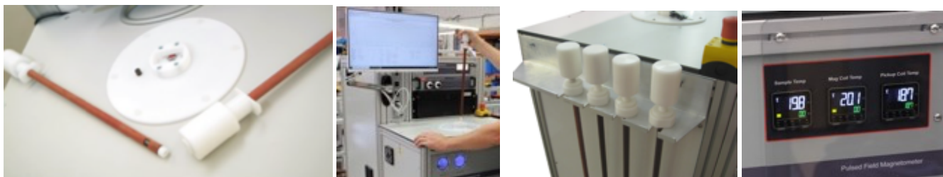
Above: PFM08-10 AT MH sample holder stick, a PFM08-10 AT MH in operation. Samples stick storage on the side of the PFM08-10 AT/HT MH and sample temperature measurement displays.
