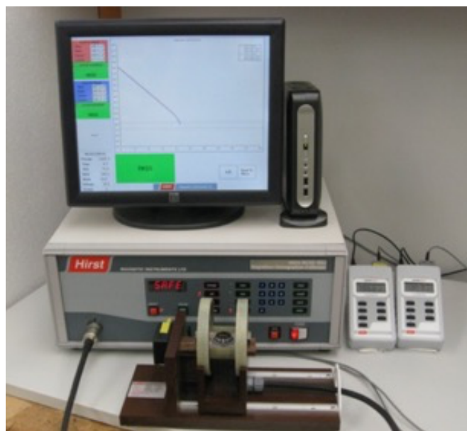
MCSD200J magnetiser and custom fixture and 2 gaussmeter probes with GM08s used for precision navigation sensor production.
