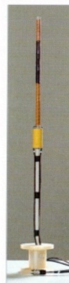
PFM02 inductive pickup coil assembly and adjustment mechanism.
