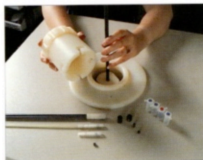
Various sizes of sample can be positioned in the appropriate sample holder. These are fitted to the sample rod and inserted into the Measurement Chamber. (Manual sample system)
