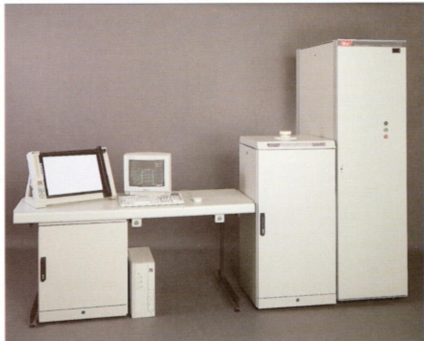
Full loop measurements of sintered and bonded Neodymium Iron Boron and Barium Ferrite.
