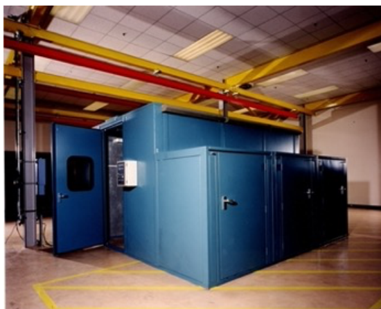
Custom production enclosure containing a second generation M3000-100kj magnetiser.
