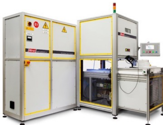
A third generation M3000-40kj Magnetiser with custom skewed multipole fixture for IPM motor applications with IFM06 fluxmeter and embedded Gaussmeter feedback.
