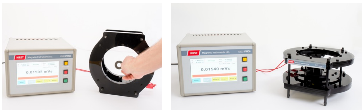
Above is a HH-150 mounted (left) on its side and vertically (right) with the standard magnet sample table (included). Note the IFM06 fluxmeter is sold separately.
