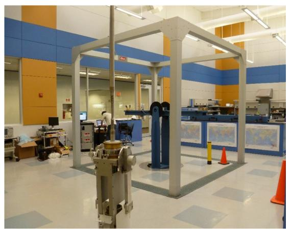
The image above shows the cube in its final application, complete with the equipment calibration rig inside. The cube sits within a trench, so that there is easy access to the calibration rig, and personnel can easily move in and out of the area. The cube is controlled via the instrumentation which sits outside in racks.
