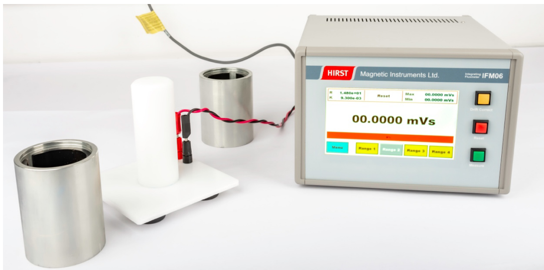
Custom sense coil for a 2 pole PMDC magnet assembly connected to a IFM06 fluxmeter
