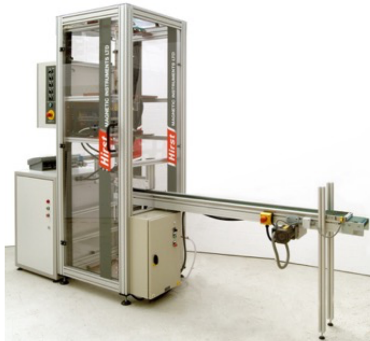
Toy production – a M4k workstation with custom fixtures and high throughput integrated conveyor system with 4 parallel lines on a 1.2 second duty cycle running 24hrs a day.
