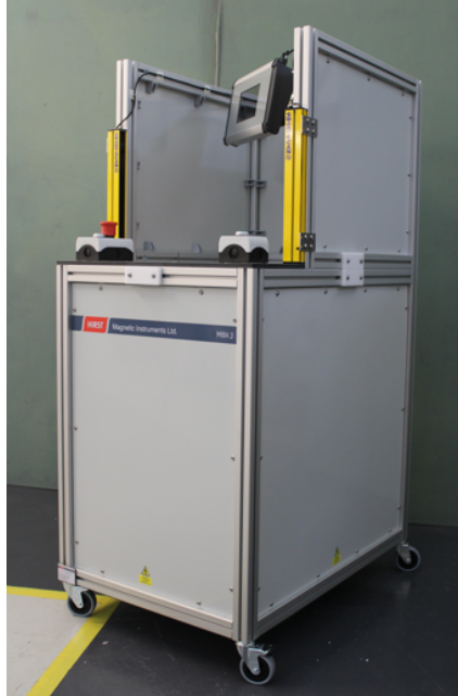
M8k magnetiser workstation with 2 pole custom fixture for loudspeaker production with light guard safety enclosure.
