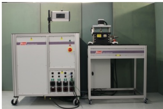
Custom M12kj magnetiser workstation with custom fixture for a valve actuator application.
