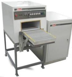
Custom demagnetisation system with conveyer feed front and back.
