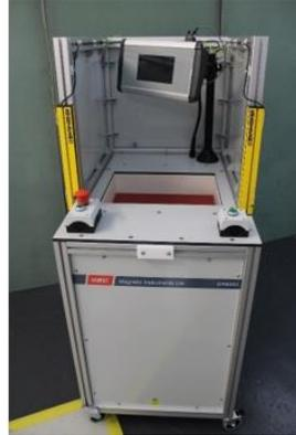
DM4kJ de-magnetiser workstation with tray de-magnetisers for medical needles. Each tray contains about 250k parts, with each shot achieving <math><5</math> Gauss on all parts.
