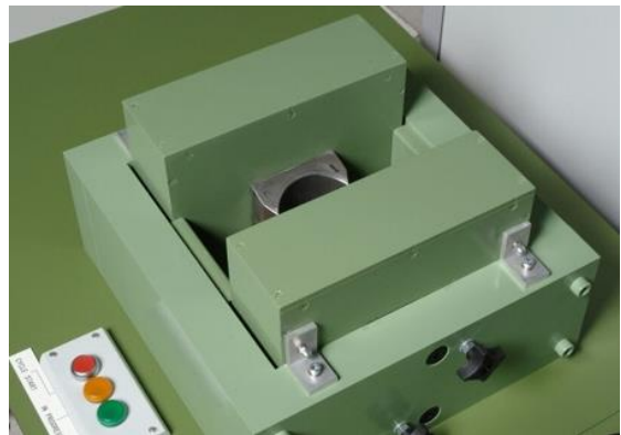
2 pole custom fixture for SPM motor production
