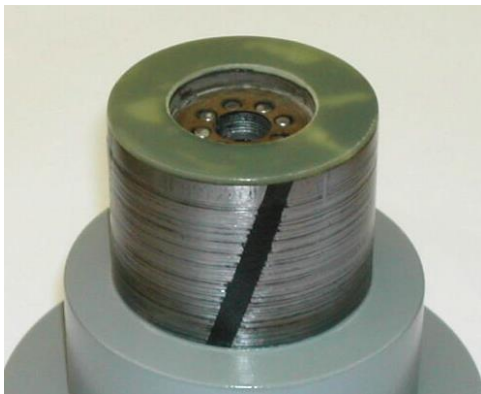
Custom 4 pole skew fixture for medium size IPM motor
