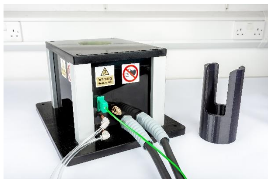
Custom benchtop fixture for use for 100mm diameter magnets used in actuators in medical industry fixture us water cooled and features temperature monitoring
