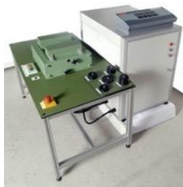
Above a M12kJ workstation with custom fixture for medium IPM motor production
