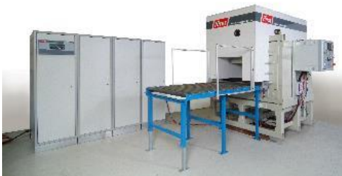
M800-400kJ Magnetising system with handling equipment and custom 2 pole fixture for magnets used in the recycling industry weighing up to 1 Tonne
