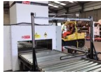
A custom 2 pole fixture in use with a M800-400kJ magnetiser for manufacturing 1.4 tonne magnets for use in recycling applications
