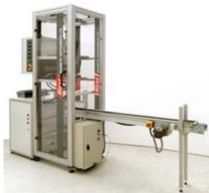
M4kj workstation with custom fixture and high throughput conveyor system with 1.2 second duty cycle running 24hrs a day with 4 parallel production lines
