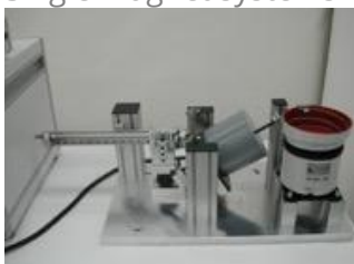
Custom 2 pole fixture for single magnet piece manufacture
