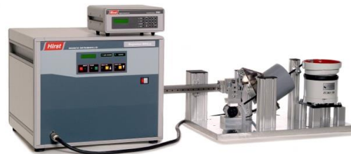
MCSD-500J and IFM02 fluxmeter running automated hopper-based sensor magnetiser
