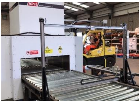
Above a custom 2 pole fixture for use with a M800-400kj magnetiser for manufacturing 1.4 tonne magnets for use in recycling applications
