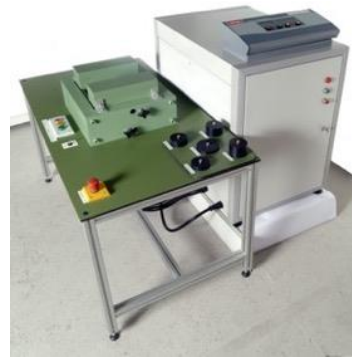
Above a M12kj workstation with custom fixture for medium IPM motor production – semi-automatic system
