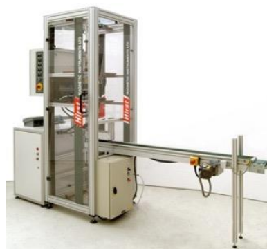
M4kj workstation with custom fixture and high throughput conveyor system with 1.2 second duty cycle running 24hrs a day – 4 parallel lines
