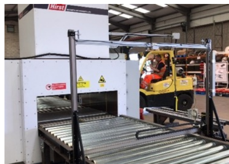
Above a custom 2 pole fixture for use with a M800-400kj magnetiser for manufacturing 1.4 tonne magnets for use in recycling applications
