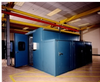
Above a custom production enclosure containing a M3000-100kj magnetiser
