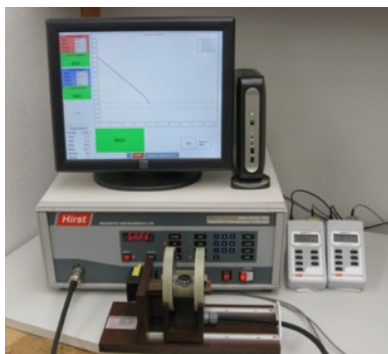
MCSD200J magnetiser and custom fixture and 2 gaussmeter probes GM08 used for navigation sensor production
