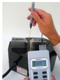
GM08 used to test J2a fixture field
