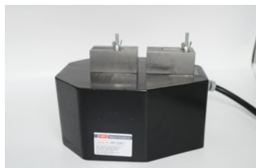
Above J2A 2 pole axial fixture Up to 500J for sensor applications
