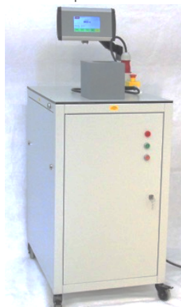
M8kj magnetiser workstation with 2 pole custom fixture for loudspeaker production
