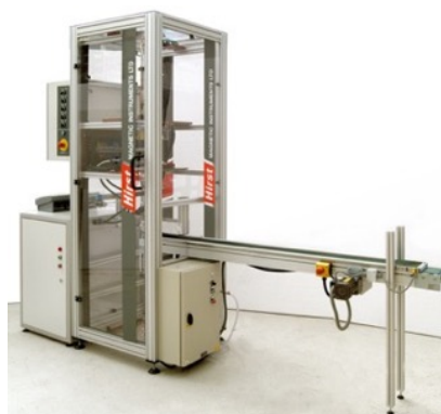
M4kj workstation with custom fixture and high throughput conveyor system with 1.2 second duty cycle running 24hrs a day
