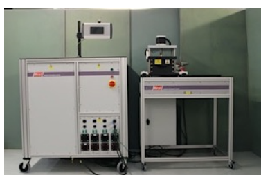
A custom M12kj magnetiser workstation with custom fixture for valve actuator application
