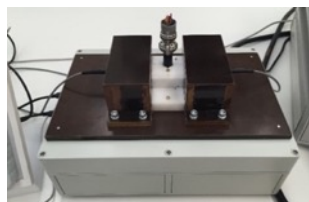
Gaussmeter probes integrated into a calibration fixture for a sensor application
