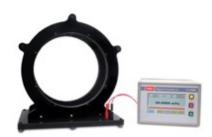
Above an IFM06 with a Hirst 300mm (HH-300) Helmholtz coil pair used for permanent magnet measurement and quality control applications see Hirst Helmholtz coil selection guide and application note.
