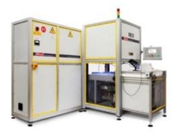
Above an IFM06 used as a production controller providing feedback to control a Hirst M40kJ Magnetiser with a custom Magnetising fixture in an automotive EV motor production application.
