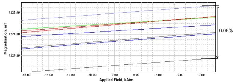
The above graphs show a selection of measurements that were taken over a 37 minute period. During the test the magnet sample was fully removed and inserted from the system for each test and this still resulted in a repeatability of better than +/- 0.08 % for J and H. The results are also tabulated in the table below. This is a selection of measurements over the 37 minute period, the system its self is capable of a cycle time of 12 seconds with the same level of repeatability.
